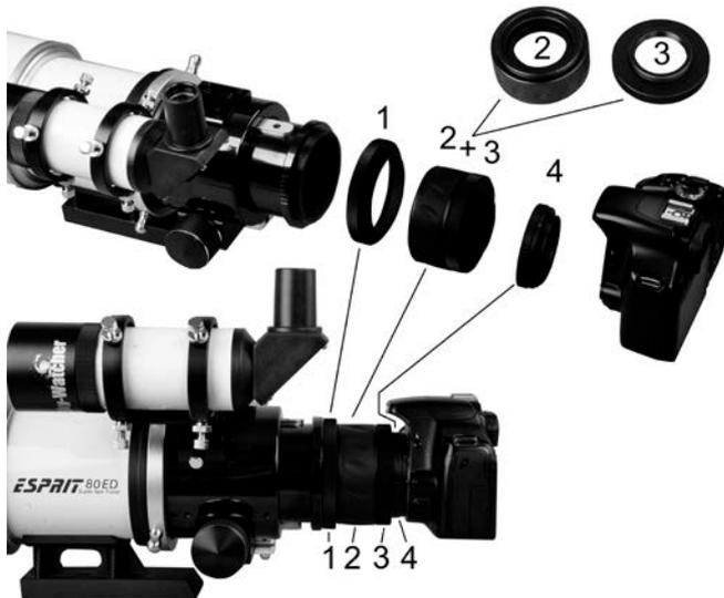
1. Screw the drawtube adaptor (1) at the end of the focus tube.
