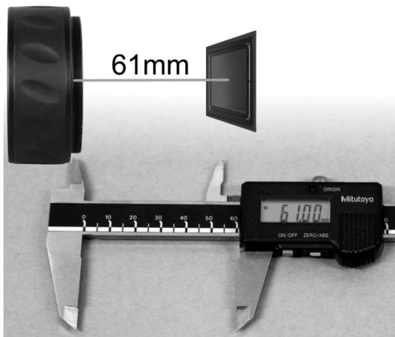
The 61mm distance is measured from the edge marking the start of the male thread on the field flattener, to the CCD sensor (See picture on the left).
