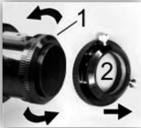
Before installing the field flattener onto the drawtube of the focuser, the 2" ring adaptor (2) needs to be unscrewed and removed.
