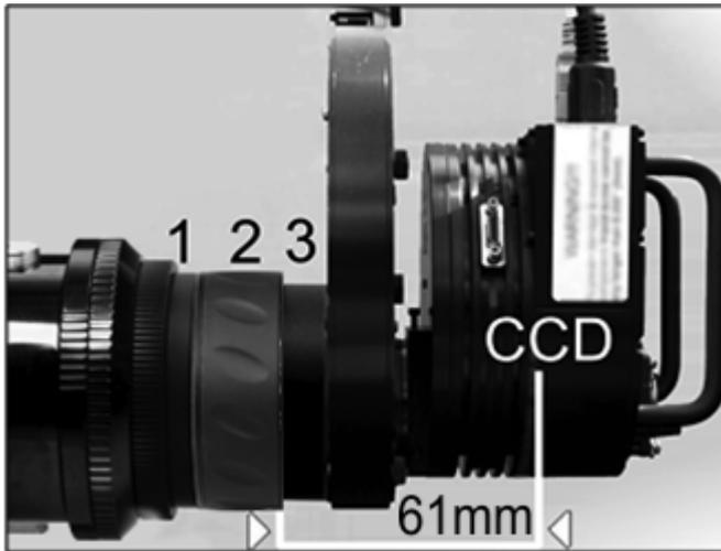
1. Screw the drawtube adaptor (1) at the end of the focus tube.
